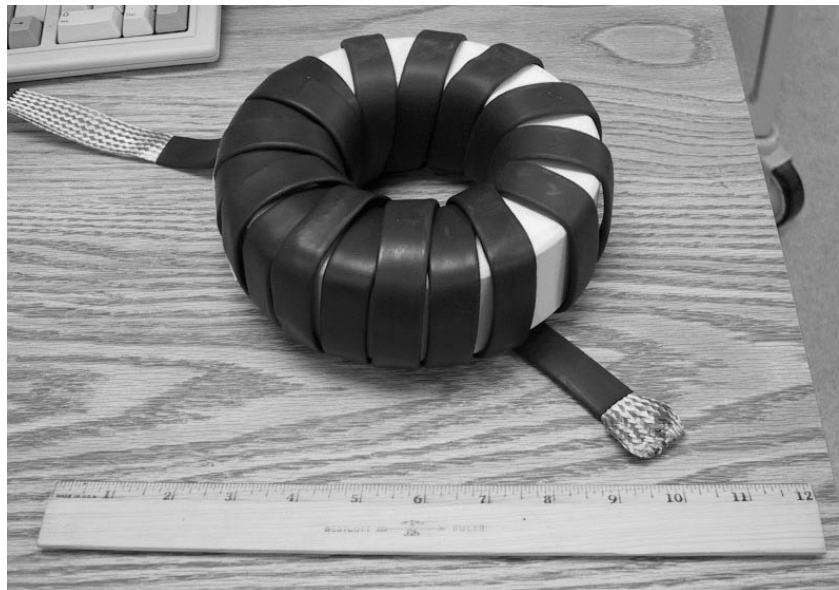
Figure 9. Input inductor for 10 kW inverter system.
